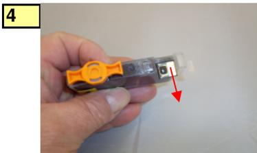
**4** Remove the chip carrier (with chip on it) from the empty cartridge "Sideways"
