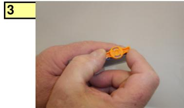
**3** Remove protecting clip by rotating anti-clockwise
